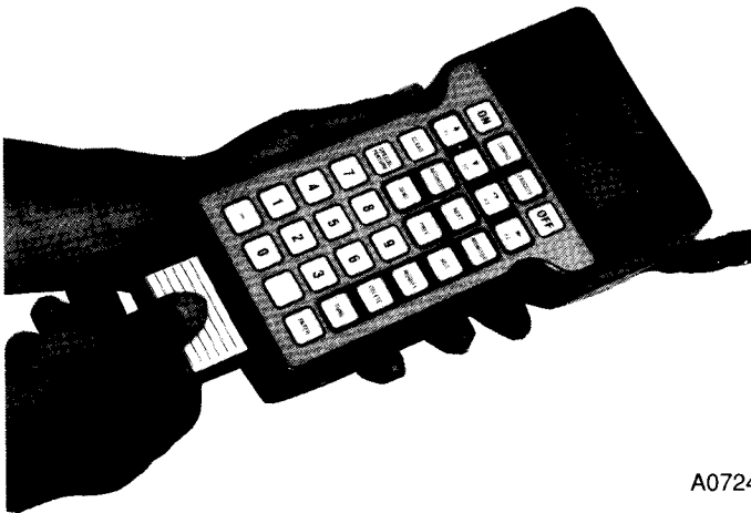
FIGURE 6 – Installing and Removing the CTT02 Cartridge
